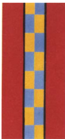
Figure 4. The cellular texture of the nematic phase viewed at different orientations between crossed polarizers with a 1\lambda plate inserted at 45^\circ .
